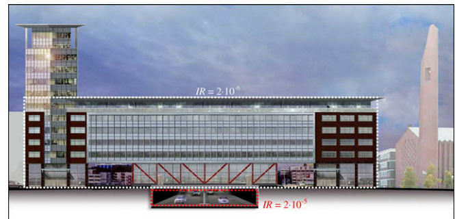
Fig. 9. The (schematic) IR contours in the third dimension for Bos and Lommer building (source artist impression: www.multivastgoed.nl ).
